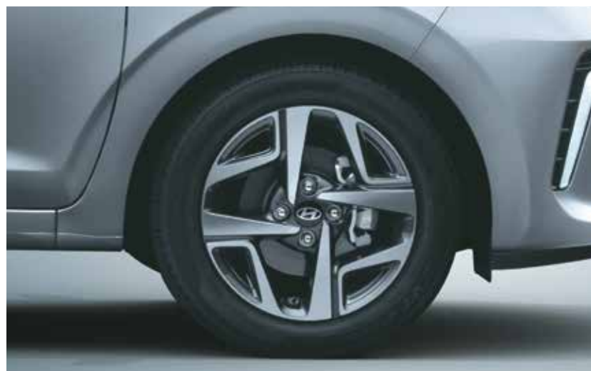
R15 (D = 380.2 mm) Diamond cut alloy wheels
